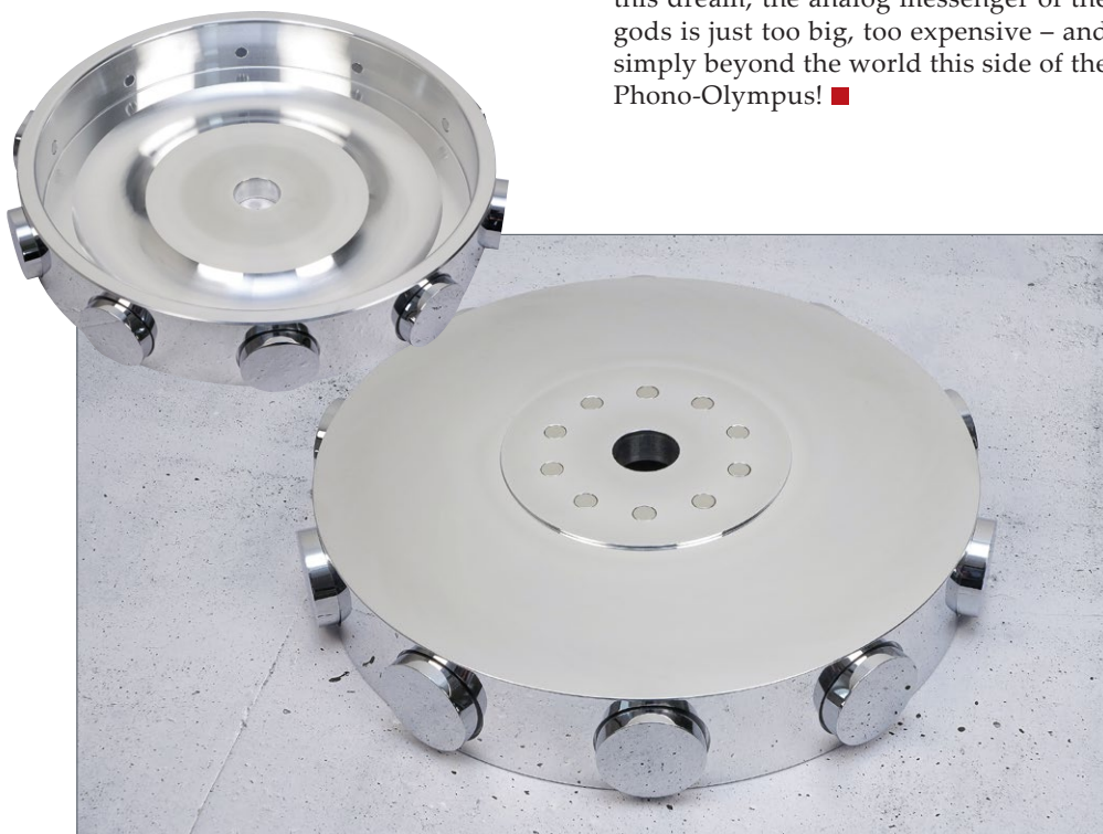
The aluminum sub-platter, which is also impeccably worked inside (above), has the same number of magnets as the drive disc. Chrome-plated brass weights at the outer edge increase its mass.
