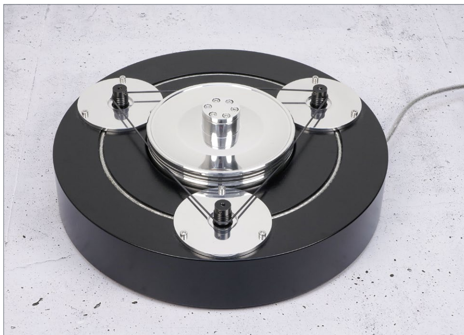
The drive unit with the three motors is made of solid aluminum. In sum, the three drive belts exert no lateral forces on the bearing, so that it runs without tilting.
