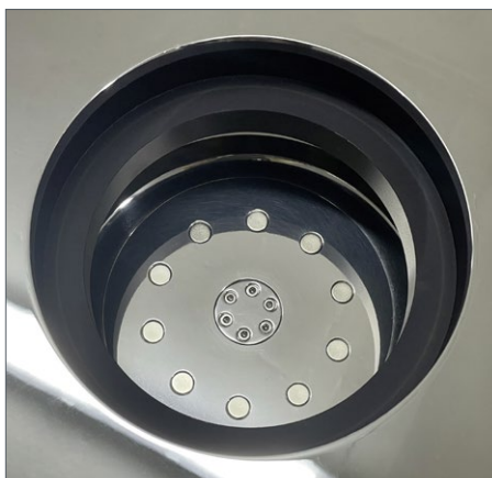
Before mounting the platter, you look at the drive disc fitted with magnets.
