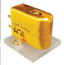
Microline also has a contact surface of only 0.08 mm (80  $\mu$ m), placed on a 0.22 mm diamond cantilever. The magnetic circuit uses a combination of soft iron and samarium cobalt on a 2.5 mm sapphire base on a cross-coil support. With an internal impedance of 4 ohms, it offers an ultra-low output voltage of 0.3 mV (at 1 kHz) and weighs only 8.7 g; it is positioned like the previous one at €15,000.
